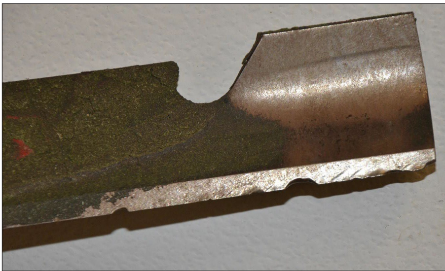
Figure 1. Dull mower blades increase mower fuel usage and potential for disease in grass plants.
