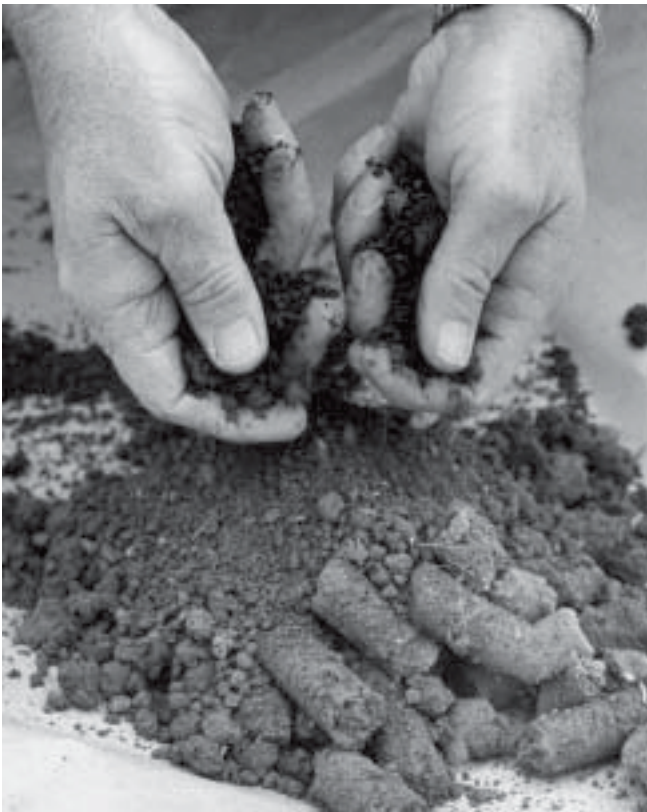
Figure 4. Break up clods while a sample is moist, and spread out to air dry in a clean area.
