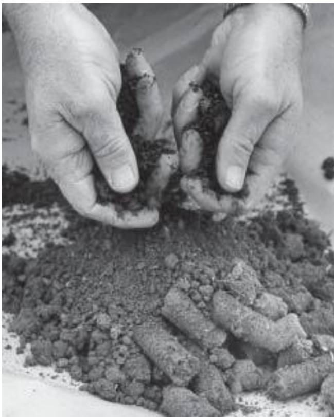
Figure 4. Break up clods while a sample is moist, and spread out to air dry in a clean area.
